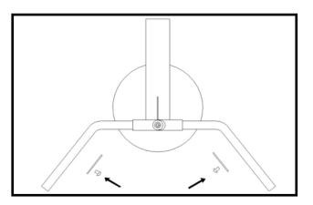
**2.** Fit left hand arm into channel until roll pin touches channel as shown. (**ARROW ON PICTURE**)
